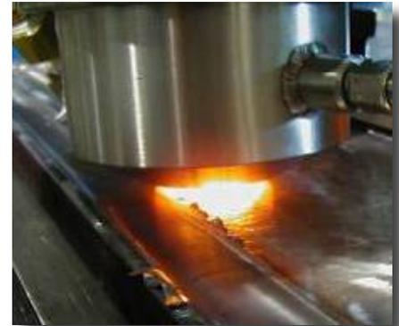
*Friction stir welding of steel*
